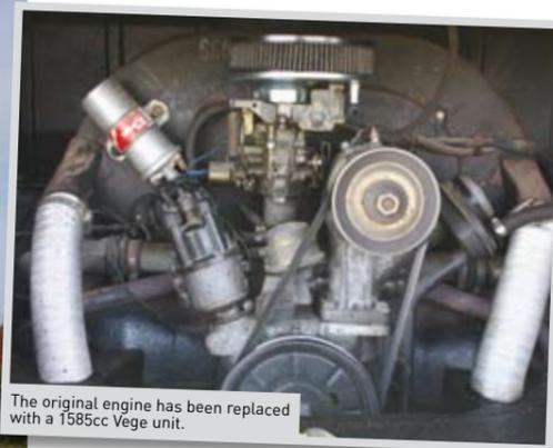
The original engine has been replaced with a 1585cc Vege unit.
