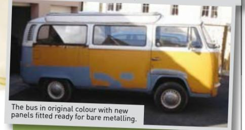
The bus in original colour with new panels fitted ready for bare metalling.
